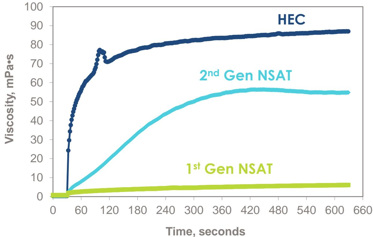
2<sup>nd</sup> Gen NSAT viscosity recovery profile allows leveling to proceed while preventing dripping
